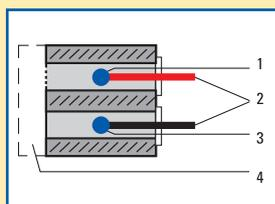
The inert element is for compensating the temperature and conductivity of the test gas.
